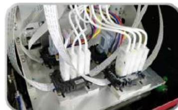
4 printhead, faster, higher accuracy
